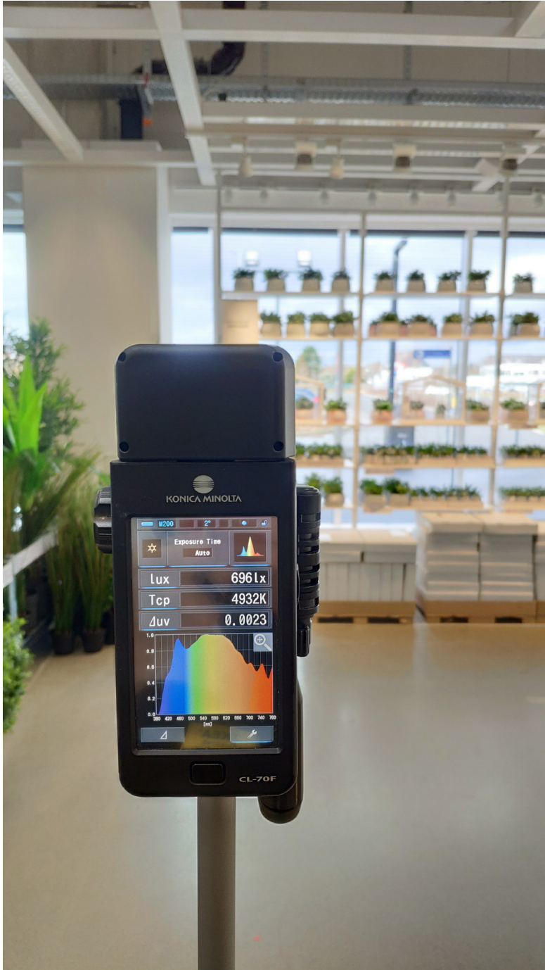
Figure 12.4 A spectroradiometer measuring vertical irradiance. The normalized SPD, the vertical illuminance, the CCT and Duv of the incident light is shown on the screen. The raw data can be saved and used in circadian toolboxes for calculating the relative circadian metrics. Image: Niko Gentile.
