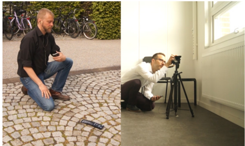
Figure 12.2 The two surveyors are measuring daylight factors while being in contact through the phone. Left: outdoor measurement of global horizontal diffuse illuminance. Right: indoor measurement of horizontal illuminance, with lux meter positioned on a tripod at 0.8 m height. Image: Niko Gentile.
