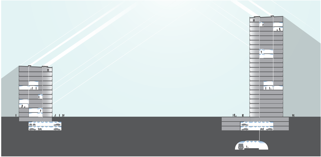
Figure 10.22 Fiber optic system, from Parans. Illustration: Parans Solar Lighting AB.
