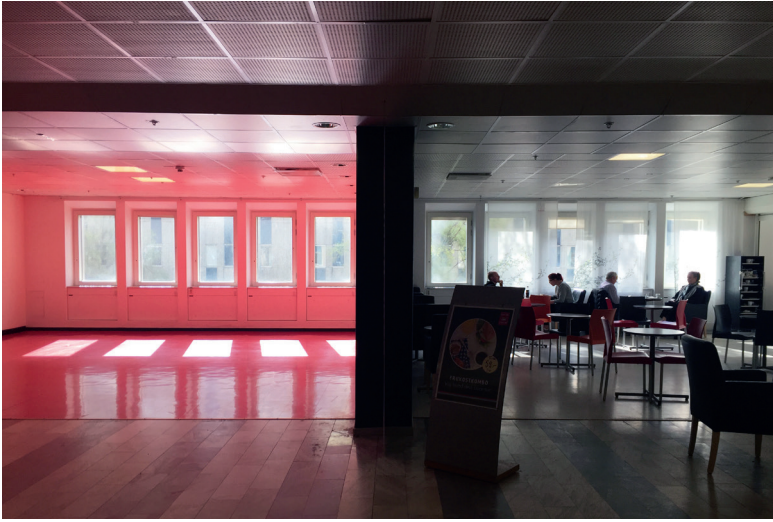
Figure 3.3 Huddinge hospital, Sweden. Two adjacent rooms with the same (white) colour for walls and ceiling but different colours for the floor. Photo: Malin Alenius.
